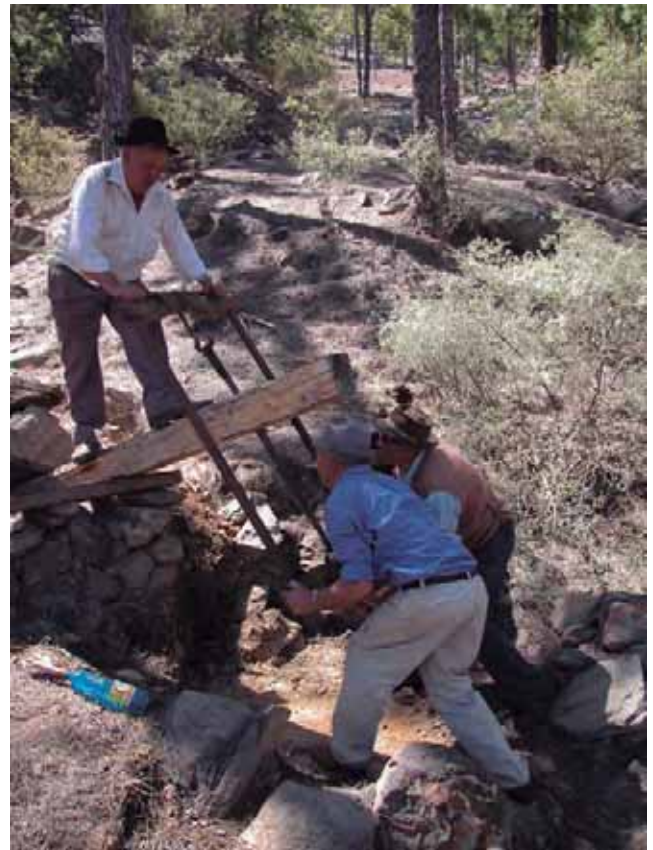
Figure 2.a.206. The "serrote", one of the traditional tools used for cutting and clearing wood. © Julio Cuenca
