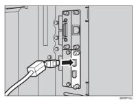
Plug the other end of the cable into the connector on the computer's interface.
